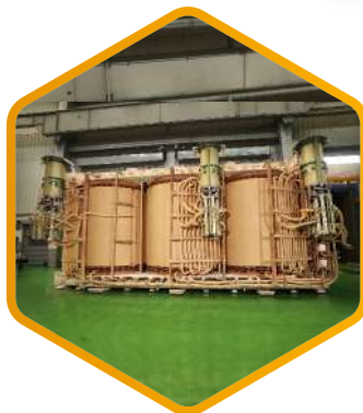
500MVA, 400kV Transformer Core Building Assembly
