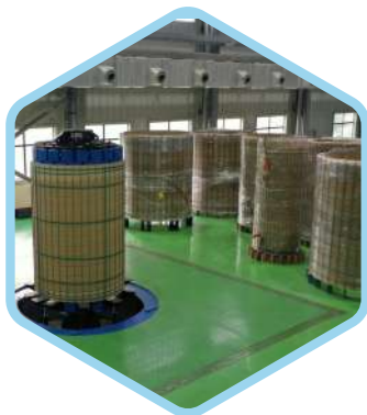
Coil Winding of 500MVA, 400kV Transformer on Vertical Winding Machine
